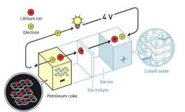
• Akira Yoshino: The first commercially viable lithium-ion battery was developed by him in 1991. He replaced lithium anode with petroleum coke anode, which drew Li-ions towards it from the Lithium Cobalt oxide cathode.
